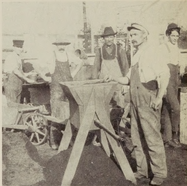
At Poehlman's about the turn of the century. Geo. J. Ball at extreme left. Note hand cranked soil grinder.
